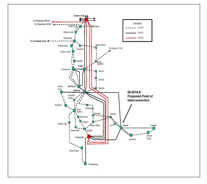
Figure 1 Boone Substation and Surrounding Transmission System
